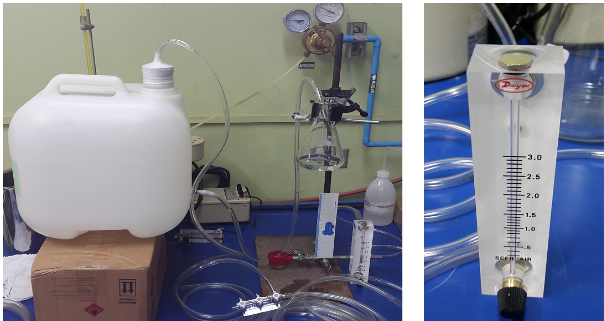
Figure 2: Left) Pressurized container which simulates the pressure in a biodigester and is being used to estimate the flowrate of the biogas. Right) Enlarged picture of a laboratory type gasflowmeter.
